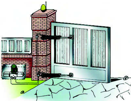
Double mount where 2 rams are required to open/close a single gate
